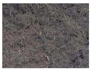
This BMP consists of applying a mixture of shredded wood mulch, bark, or compost to bare soil to reduce runoff, increase infiltration, and reduce erosion due to wind or rainfall impact. Wood mulch provides temporary or short-term soil stabilization. This material should be applied to exposed soil beneath the existing tree canopy along the eastern edge of the facility and adjacent to Arnold Road.
