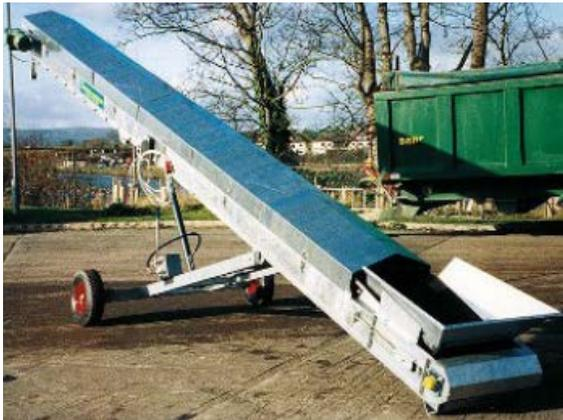
This BMP consist of covering dust generating equipment on-site or establishing a non-natural barrier to prevent dust contamination. Equipment coverings can range from covering individual components of processing equipment (such as covered conveyor belts, hoppers, etc.) to constructing a screen or fence barrier to limit off-site transport.
