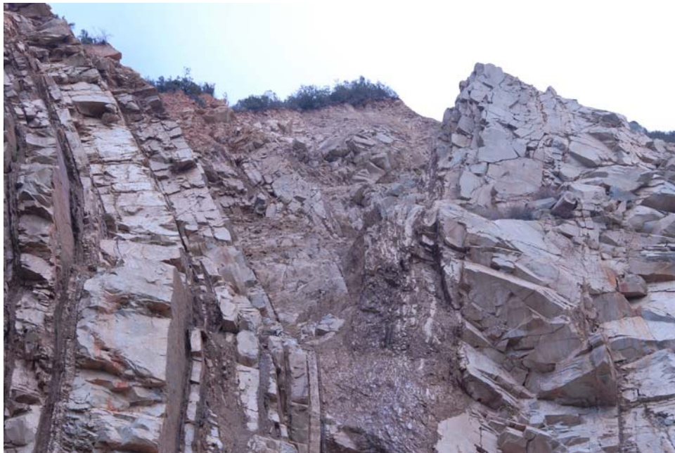
Photo 8: A fault zone in the upper part of Domain A (triangle shape). The Triangle Zone (Photo 6) is located up-slope of this area.
