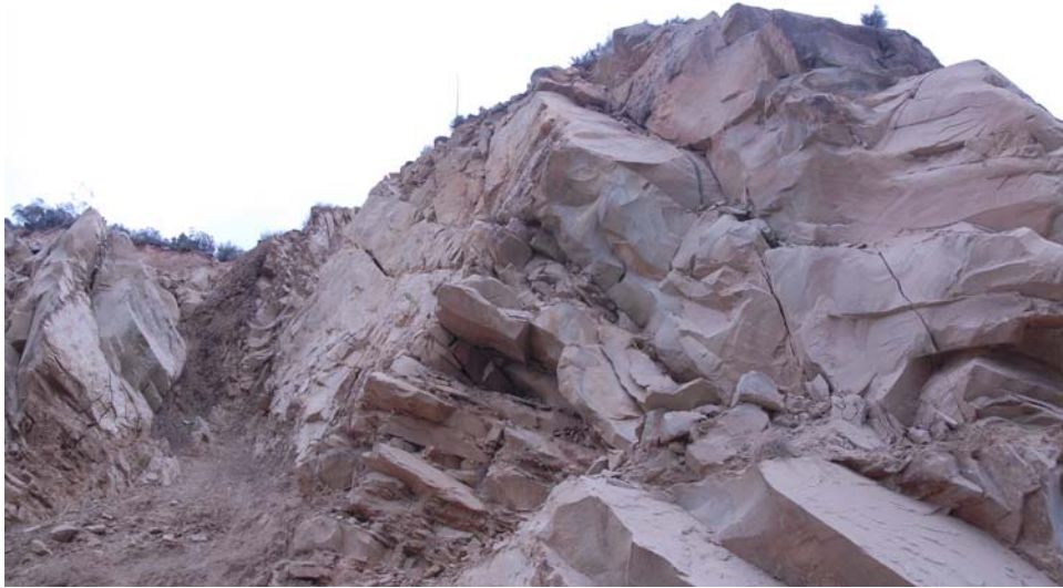
Photo 5: Thick sandstone beds in Domain C (at the south end of the quarry). This area was blasted. Note the wider spacing of the joints. The valley on the left is likely a fault zone. It is unknown if it is a bedding plane fault.
