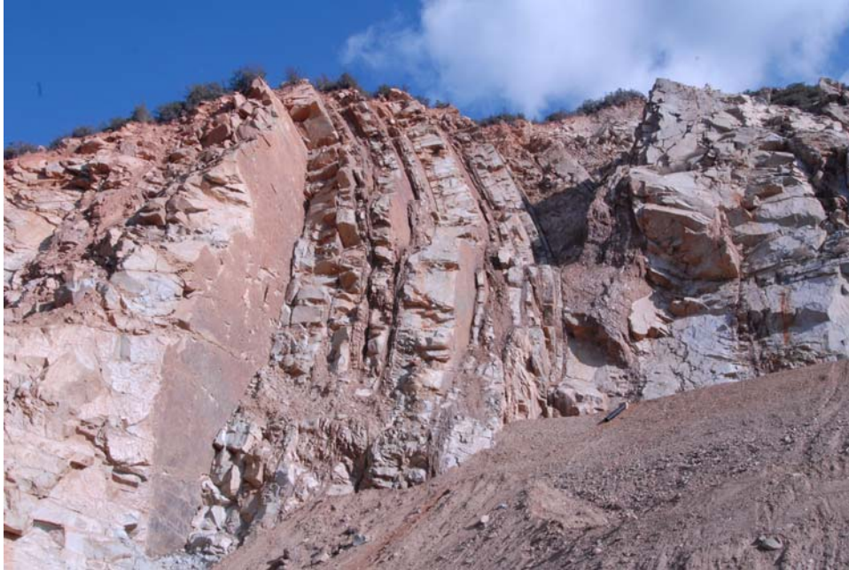
Photo 3: Sandstone beds at the northern end of the quarry (Domain A). There are thin siltstone beds between most of the sandstone beds. Even though jointing is pervasive, few joints extend across multiple beds.
