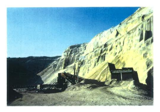
Photo No. 4 View of active mining area. Material is pushed down the slope and loaded into hopper for transport by conveyor belt.
