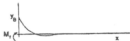
Fig. 18. Pile deflection produced by moment applied at mud line.
