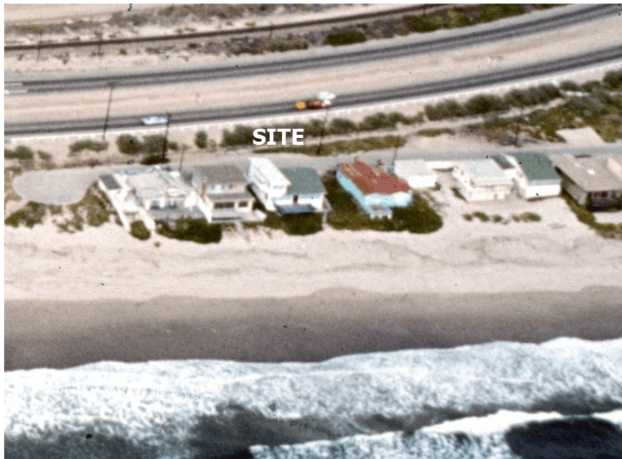
Photograph 2. Subject site and shoreline in 1972. Note that the beach width has not change over the ~50 year time period between Photograph 1 and Photograph 2.
