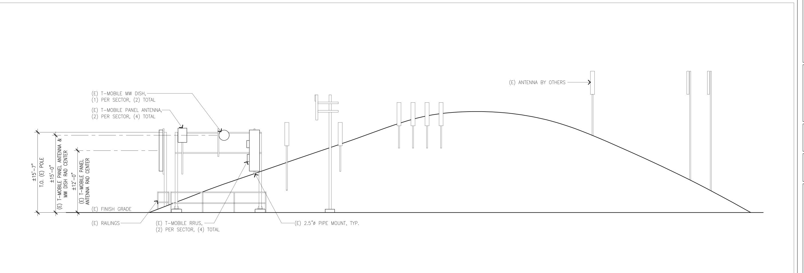
SCALE: 3/16"=1'-0" **EXISTING SOUTHEAST ELEVATION** —(E) ANTENNA BY OTHERS —(E) T—MOBILE MW DISH, (1) PER SECTOR, (2) TOTAL —(E) T-MOBILE PANEL ANTENNA, (2) PER SECTOR, (4) TOTAL (E) FINISH GRADE (E) 2.5" PIPE MOUNT, TYP.— (E) T-MOBILE RRUS, — —(E) RAILINGS (2) PER SECTOR, (4) TOTAL
