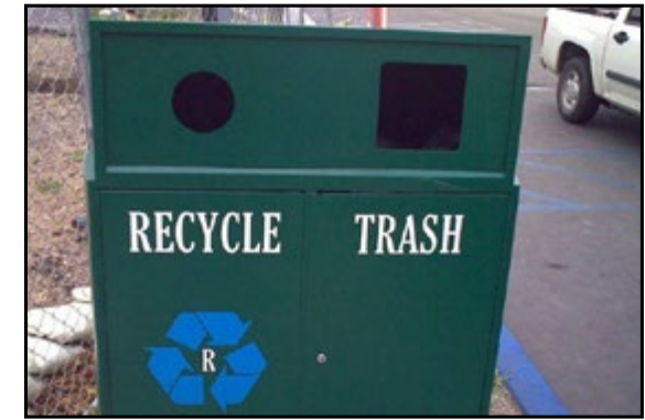
Trash and recyclables receptacles help minimize litter and keep surface water clean. 1 trash and 1 recyclables receptacle are required for the first 20 spaces, and another set for every 80 spaces thereafter. Sec. 8108-5.14
