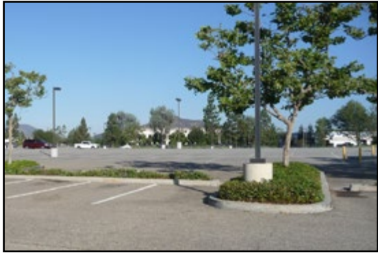
Light poles MAY NOT be located in finger planters (as pictured above), end row planters (below) or tree wells.
