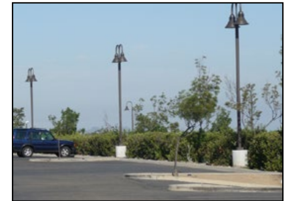
Light poles MAY be located in perimeter planters (above) and in strip planters between parking rows (below). Sec. 8108-5.12(c)
