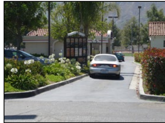
To prevent pedestrian interference, drive-through lanes must not be located between the street and the main building entrance.
