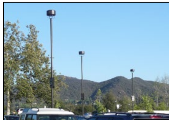
Full cut-off lighting prevents light from going above the horizontal plane in order to minimize lighting of the dark night sky. All new lighting fixtures in parking areas must be full cut-off. Sec. 8108-5.12(e)
