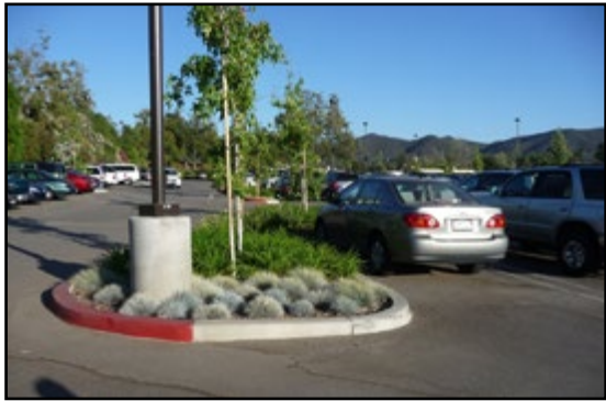
Light poles MAY NOT be located in finger planters (as pictured above), end row planters (below) or tree wells.
