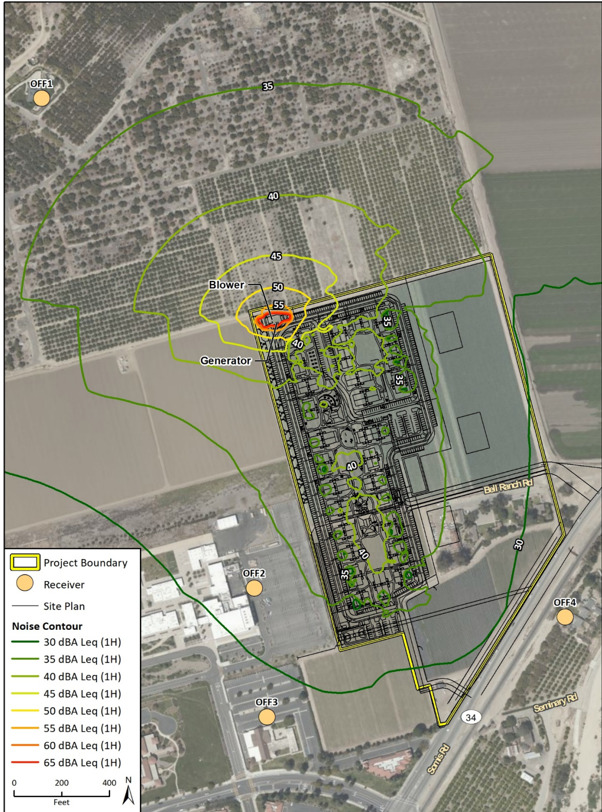
Figure 4.5-1 Off-site Receivers and Operational Noise Contours
